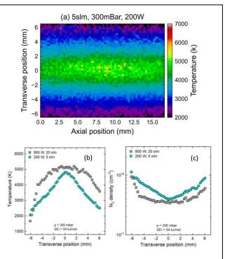
Fig. 1. a) Measured 2D image of radial cross section of reactor, showing vibrational temperature in air plasma of 200 W. b) Vibrational temperature, and c)  $N_2$  density measured in air plasma at 800 W and 200 W, SEI = 54 kJ/mol
